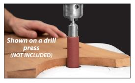
**Operation** - For optimum drum sander performance it is recommended that you move your stock back and forth across the sander. Keep steady pressure against the drum sander without applying too much force. Placing to much pressure against the drum will cause your stock to burn and may damage the drum.
